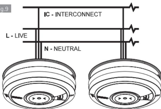
Make electrical connections as shown in Figure 9. Wiring must be installed in compliance with local regulations.
