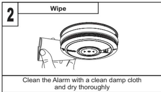
Use the narrow nozzle attachment of your vacuum cleaner to remove dust, insects and cobwebs from the sides and cover slots where the airflow enters. Clean the outside cover by occasionally wiping with a clean damp cloth then dry thoroughly with a lint free cloth. Do not use any cleaning agents, bleaches, detergents or polishes, including those in aerosol cans.
