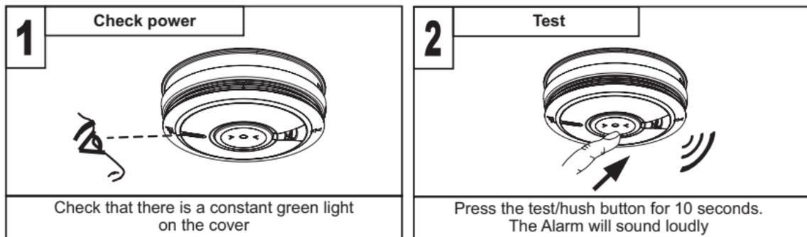
(i) Check that the **green LED power indicator** is on continuously.
